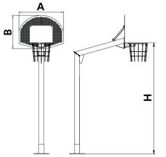
**Structure, Metal:** cylindrical post made of steel. Steel perforated board with solid square board and different support joints to avoid its deformation or damage. Double solid steel ring with room for the net.
